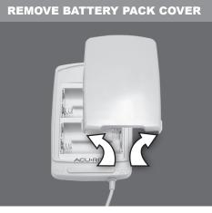
4. Remove the battery pack cover by pulling upward on the cover's tabs (away from the battery pack).
