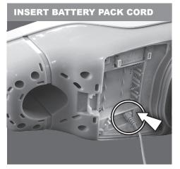
2. Plug the battery pack cord into the battery compartment AcuRite® Atlas™.
