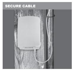
**7b.** Use the included zip ties and hardware to secure excess cable near the battery pack, leaving enough slack for a "drip-loop," preventing rain water from trailing into the battery pack. Installation is complete.
